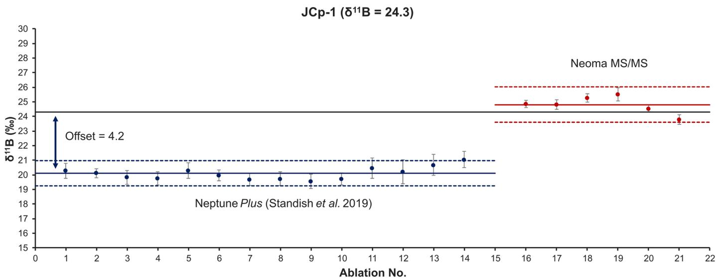
Figure 3. Comparison of boron isotopic composition of carbonate standard JCp-1 measured with the previous generation of MC-ICP-MS and with Neoma MS/MS MC-ICP-MS. All error bars are 2SE. External reproducibility (dash lines) are 2SD.
