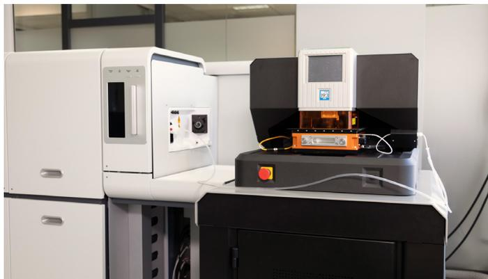
**Figure 1. Neoma MC-ICP-MS connected to ESL NWR 193 LA**
