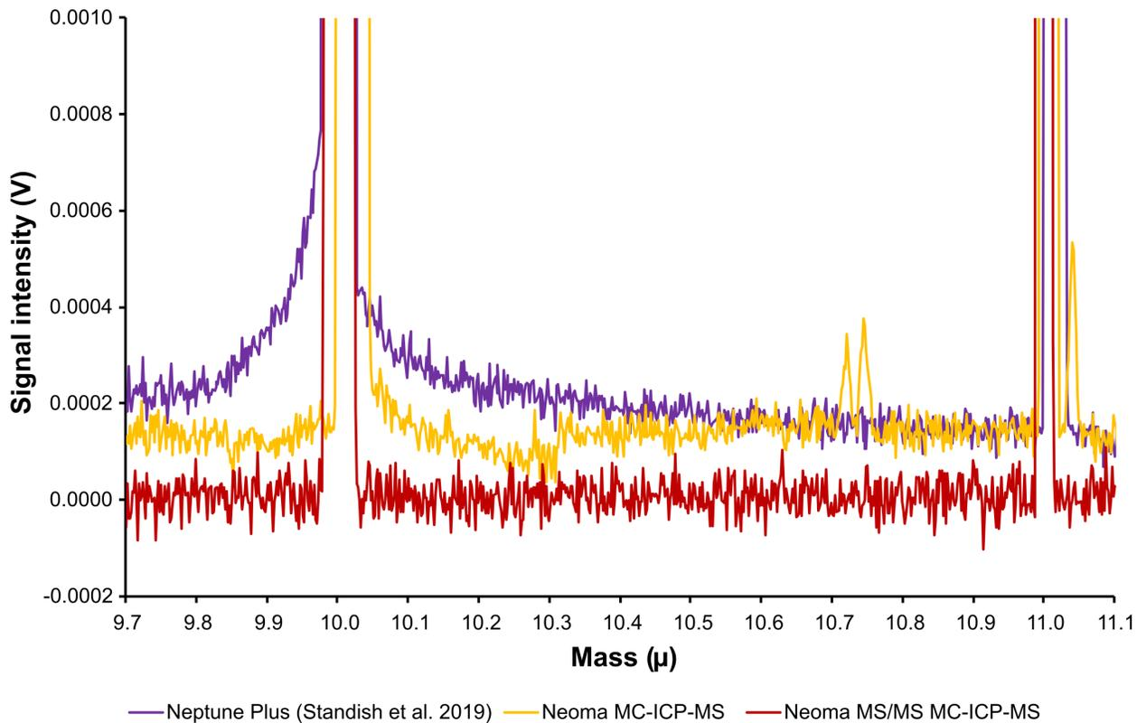
Figure 2. Mass scan across  $^{10}\text{B}$  and  $^{11}\text{B}$  when ablating the carbonate pellet JCp-1
