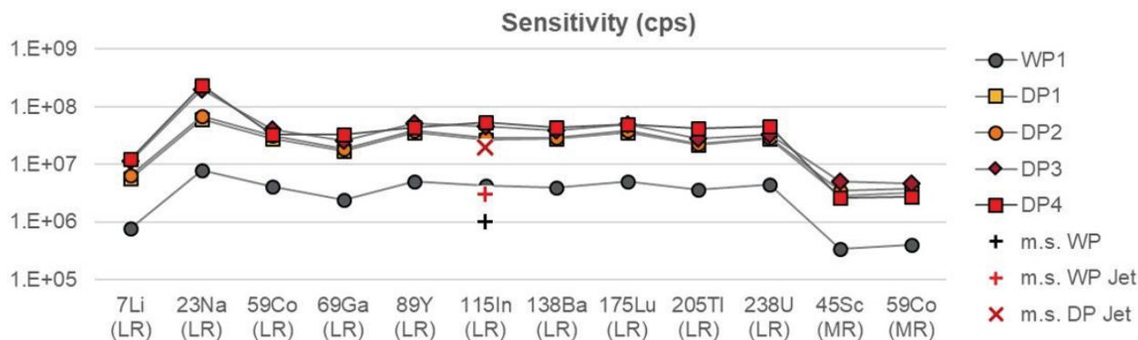
**Figure 3. Sensitivity data for experiments WP1 and DP1–DP4. Specified minimum sensitivity per 1 ppb  $^{115}\text{In}$  with standard interface in wet plasma conditions (m.s. WP) and with Jet Interface in wet and dry plasma conditions (m.s. WP Jet and m.s. DP Jet) are plotted for comparison. Note the logarithmic scale for the y-axis.**
