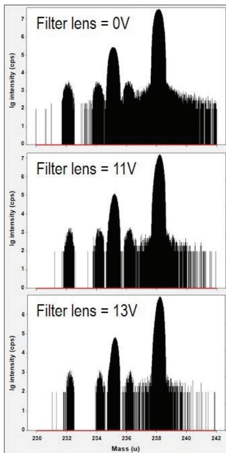
**Figure 4.** Mass scan across the 230–242 mass range at different filter lens voltages in dry plasma (experiment DP5). Note the logarithmic scale for the y-axis.
