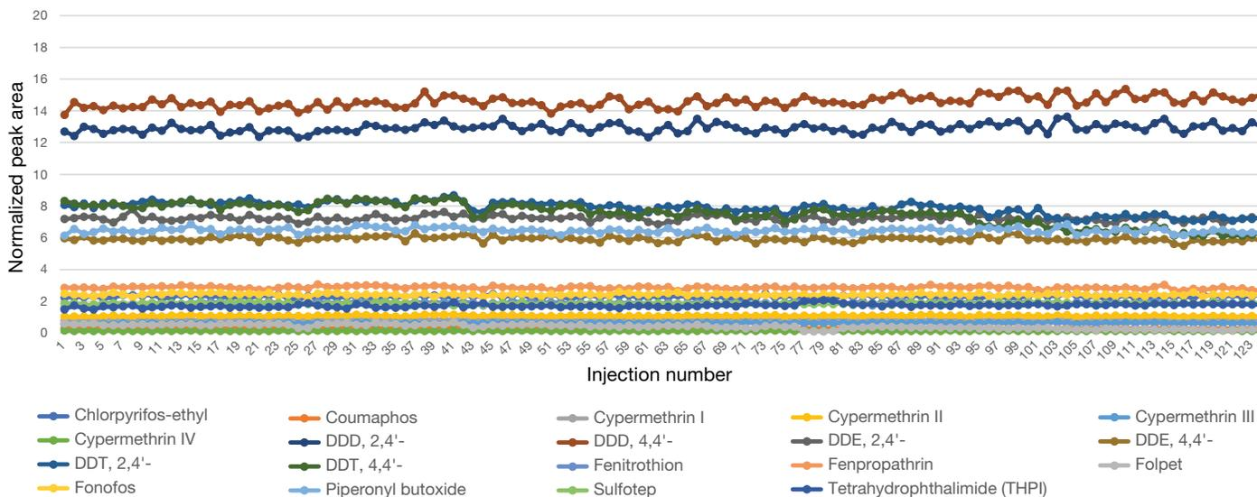
Figure 4. Normalized peak area response (analyte peak area / ISTD peak area) obtained for n=124 consecutive injections of matrix samples spiked at 50 µg/kg
