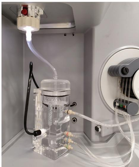
Figure 1. iCAP PRO XP ICP-OES or iCAP PRO XPS ICP-OES coupled with an integrated hydride generation kit
