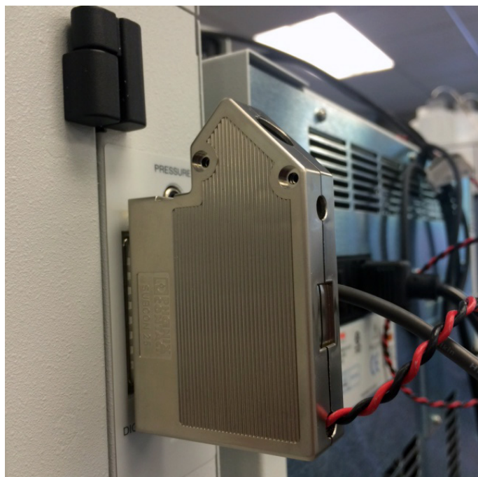
7B: Install the 25-pin connector on the back of Dionex ICS-5000+ DP module.
