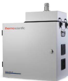
Partisol 2025i-D Dichotomous Sequential Air Sampler
