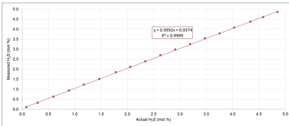
**Figure 9 Linearity plot for H<sub>2</sub>S from 800 ppm to 4.85%**
