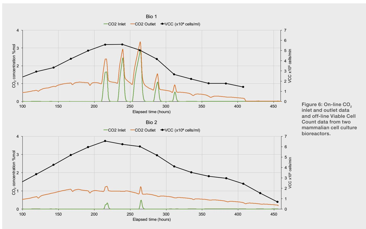
Figure 6: On-line CO<sub>2</sub> inlet and outlet data and off-line Viable Cell Count data from two mammalian cell culture bioreactors.
