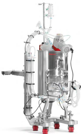
Figure 1: 50 L Thermo Scientific HyPerforma Single-Use Bioreactor (S.U.B.).
