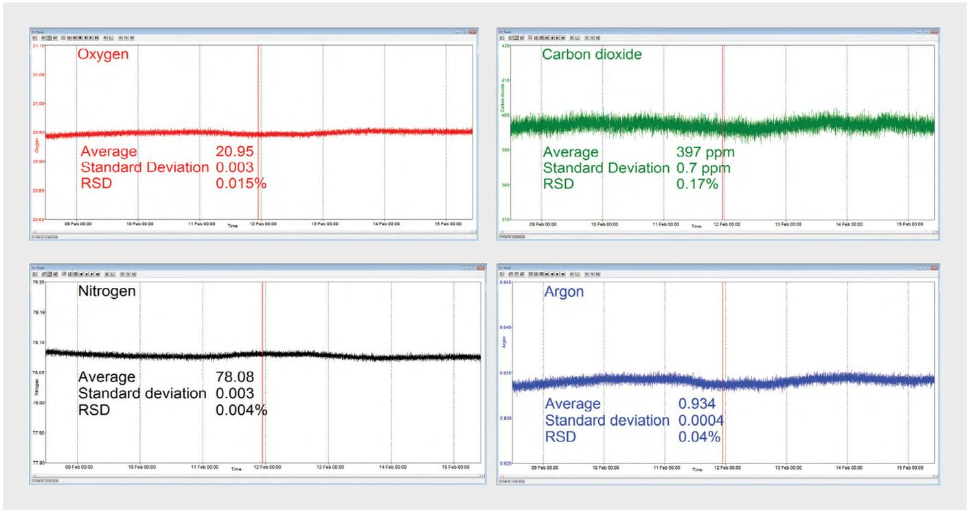
Figure 3: Long term stability data from Prima BT magnetic sector MS.
