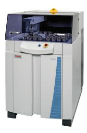
Liquid cassette recognition prevents any liquid sample to be exposed to vacuum by mistake. Over exposure safety automatically ejects a liquid sample if X-ray exposure time is too long.
