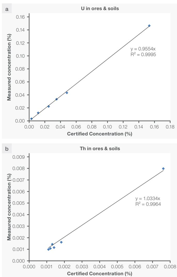
Figure 1. Verification of U and Th measurement accuracy on powdered ores and soil certified reference materials.
