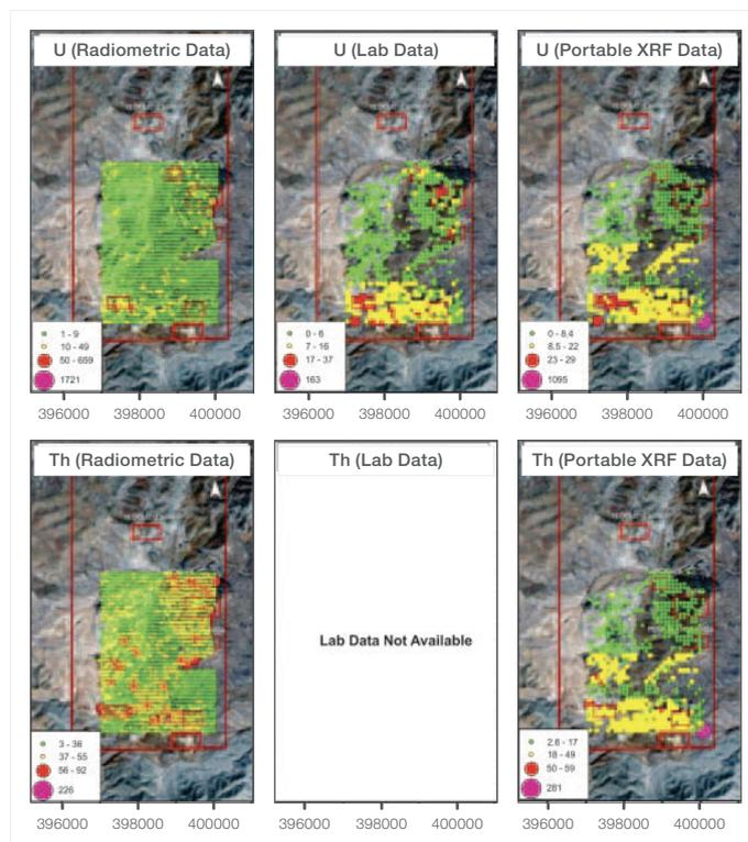
Figure 2. Geochemical map of U and Th measured by radiometry, lab, and field portable XRF.
