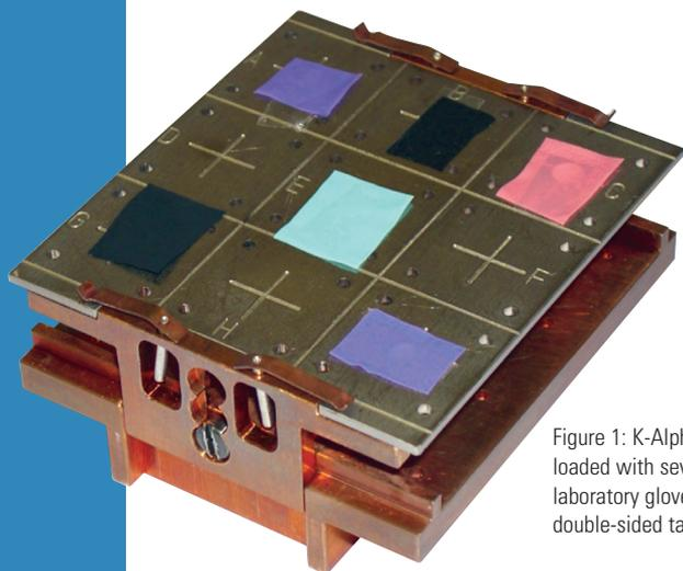
Figure 1: K-Alpha sample stage loaded with several sections of laboratory gloves mounted on double-sided tape
