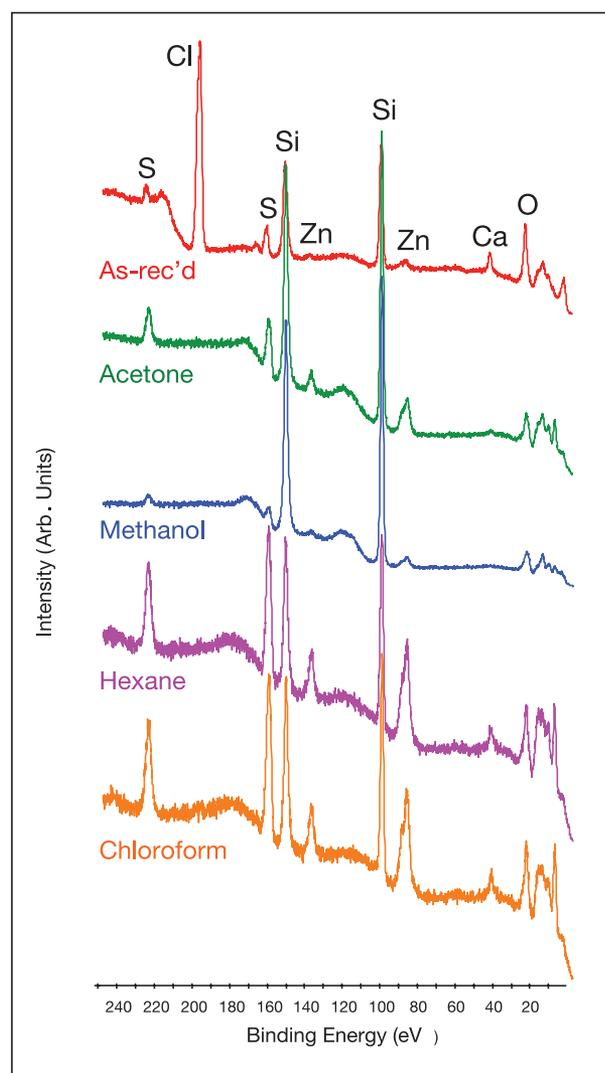
Figure 5: High resolution XPS spectra (–0–250 eV) for the as-received outer surface of Latex Glove #3 and following a 5 minute rinse in various solvents
