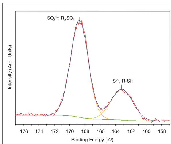
Figure 4: High resolution S 2p spectrum fitted with two peaks for the outer surface of Nitrile Glove #2
