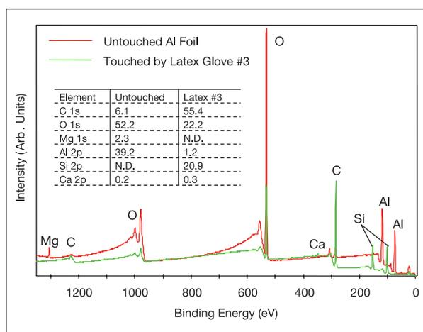
Figure 6: XPS survey spectra for clean, untouched aluminum foil and foil lightly touched by Latex Glove #3
