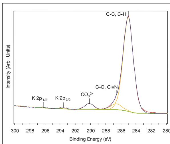
Figure 3: High resolution C 1s spectrum fitted with three peaks for the outer surface of Nitrile Glove #7. Note that trace amounts of potassium were also detected on this sample.
