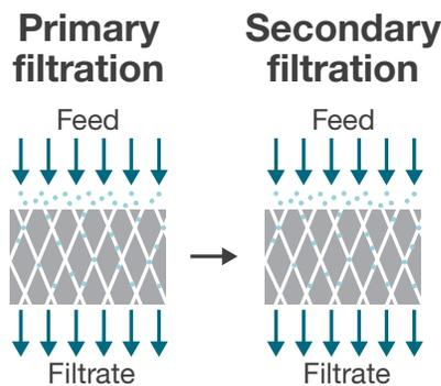
Figure 1a. Depth filtration process.
