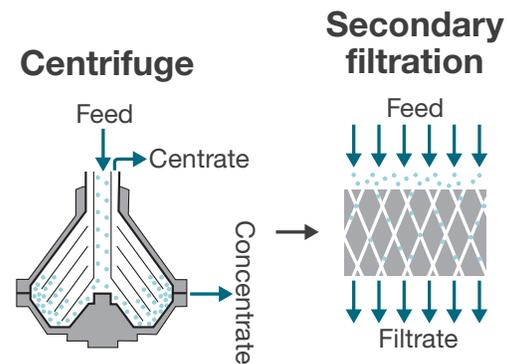
Figure 1b. Centrifugation process.
