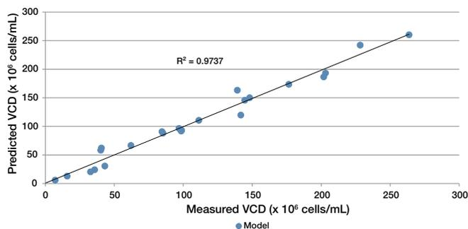
Figure 6. Model-predicted VCD vs. measured VCD.
