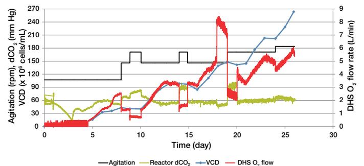
**Figure 5. Agitation,  $dCO_2$ , VCD, and oxygen flow rates for the 50 L cell culture run.**
