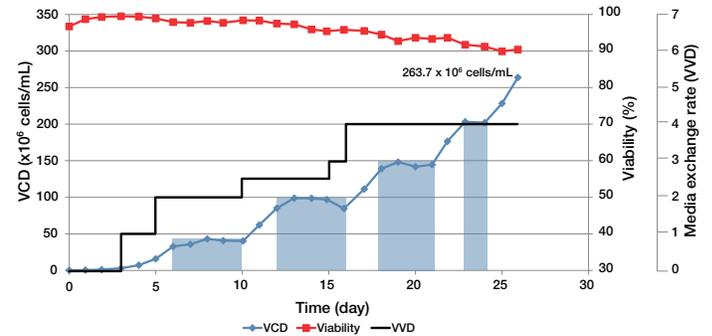
**Figure 3. VCD and viability for enhanced 50 L S.U.B. operating at 1-4 VVD. Steady-state cell density zones are highlighted.**
