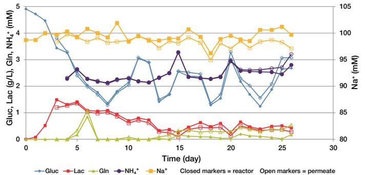
**Figure 4. Glucose (Gluc), lactate (Lac), glutamine (Gln), ammonium ( $NH_4^+$ ), and sodium ( $Na^+$ ) levels in the reactor during the culture run.**
