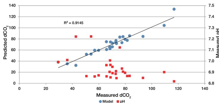
Figure 7. Model-predicted  $d\text{CO}_2$  vs. measured  $d\text{CO}_2$ .
