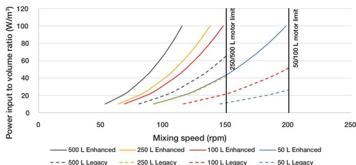
**Figure 1. Power input to volume (PIV) ratio vs. mixing speeds for legacy and enhanced S.U.B.s for perfusion from 50 L to 500 L.**
