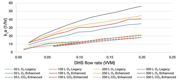
**Figure 2. Oxygen and carbon dioxide mass transfer for enhanced S.U.B.s compared to legacy systems.**
