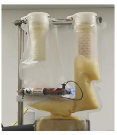
Figure 2. Pinch clamp preventing fouling of the back-up exhaust filter in case of accidental foam-out. The exhaust filter shown was intentionally foamed out to validate the effectiveness of the pinch clamp.
