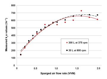
Figure 3. Oxygen delivery in the 30 L and 300 L S.U.F.s was about  $650 \pm 25$  hr<sup>-1</sup> at maximum agitation rpm and air flow rates of 2 VVM in 10 g/L NaCl in DI H<sub>2</sub>O test solution.
