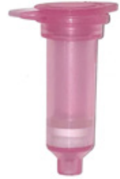
Supplier Q silica columns 100 µg binding capacity
