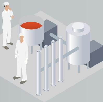
FBS is transferred to a clean room in specially designed stainless steel pipes where it undergoes 0.1  $\mu\text{m}$  triple filtration to minimize biological contaminants.
