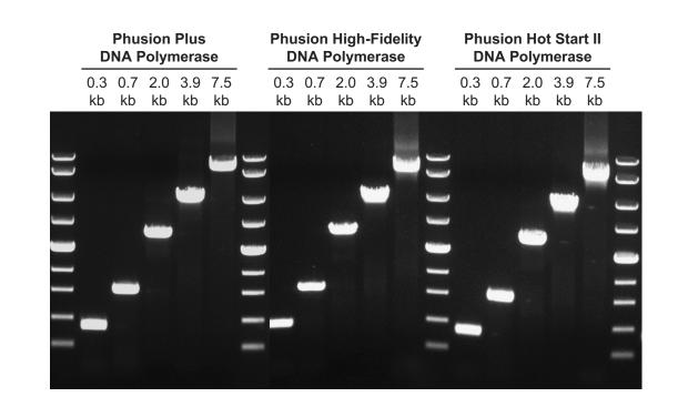
**High yields and specificity using Phusion Plus DNA Polymerase.** 0.3–7.5 kb DNA targets were amplified from 100 ng of human gDNA. The molecular weight marker is the <u>GeneRuler 1 kb Plus</u> <u>DNA Ladder</u>.
