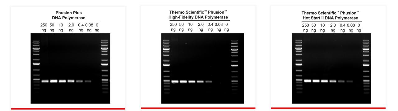
**High sensitivity of Phusion Plus DNA Polymerase.** A 0.5 kb target was amplified from different amounts of human genomic (gDNA). The molecular weight marker is the <u>Thermo Scientific<sup>™</sup> GeneRuler<sup>™</sup> 1 kb Plus DNA Ladder</u>.
