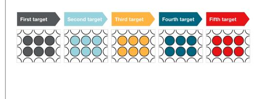
**PCR co-cycling.** Five targets of different lengths were amplified from human gDNA using a universal cycling protocol for all targets (up to 7.5 kb), with the extension time of the longest amplicon (3 min 45 sec for 7.5 kb) (left) or following separate cycling protocols with a different extension time calculated for each target (9 sec for 0.3 kb, 21 sec for 0.7 kb, 60 sec for 2 kb, 2 min for 3.9 kb, 3 min 45 sec for 7.5 kb) (right). The molecular weight marker is ZipRuler Express DNA Ladder 2.
