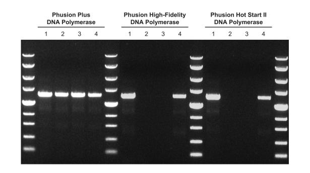
High inhibitor tolerance of Phusion Plus DNA Polymerase. A 2 kb target was amplified from 50 ng of human gDNA. The reaction mixtures contained at a final concentration of: 1—no inhibitor, 2—humic acid (0.5  $\mu$ g/mL), 3—hemin (2.5  $\mu$ M), or 4—xylan (250  $\mu$ g/mL). The molecular weight marker is the <u>GeneRuler 1 kb Plus DNA Ladder</u>.
