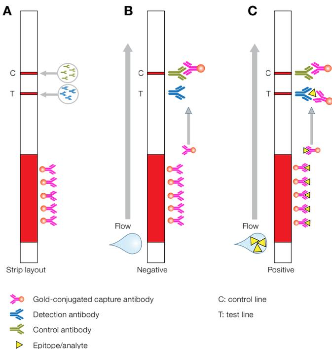
Figure 2. Pro-Detect Rapid sandwich lateral flow assay methodology.
