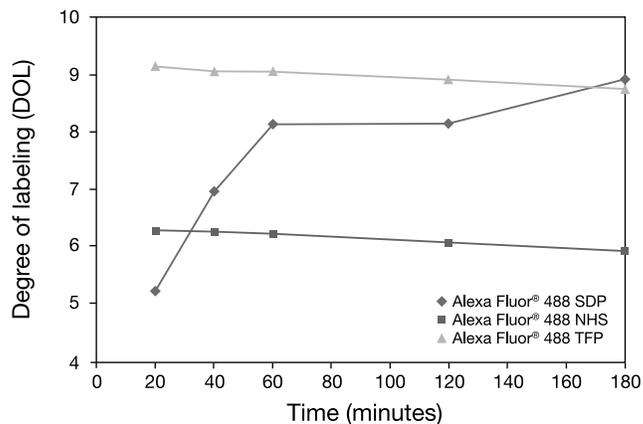
**Figure 2.** Comparison of the reaction kinetics for Alexa Fluor 488 sulfodichlorophenyl (SDP) ester, tetrafluorophenyl (TFP) and *N*-hydroxysuccinimidyl esters with goat anti-mouse (GAM) IgG antibody under standard amine-conjugation reaction conditions. After normalizing the SDP, TFP or NHS ester to 100% reactivity, they were reacted with GAM IgG antibody at a molar ratio of 12 and the resulting degree of labeling (DOL) was measured at various time points.
